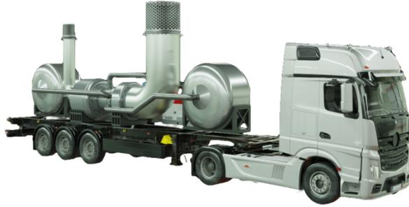
Figure 4 - NANO Nuclear Energy Inc. Internal View of Truck-Mounted Proprietary Advanced Portable Nuclear 'ZEUS' Microreactor
