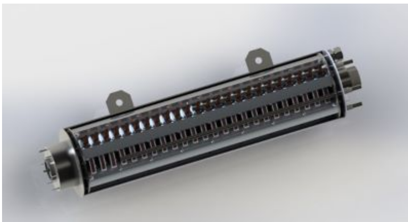
Figure 3: Annular Linear Induction Pump (ALIP) MR-24 internal structure rendering.
