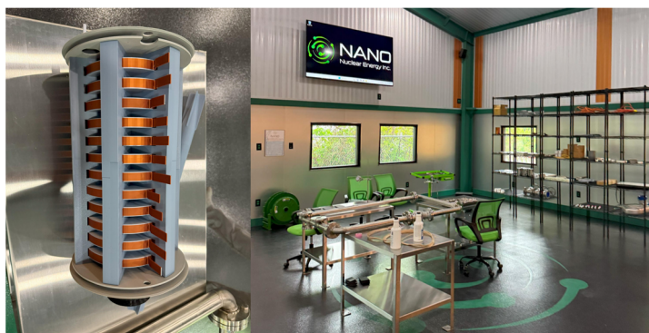
Figure 2 - Image of NANO Nuclear's Annular Linear Induction Pump (ALIP) Technology Model (left) and Liquid-Metal and Molten-Salt Test Loop (right).
