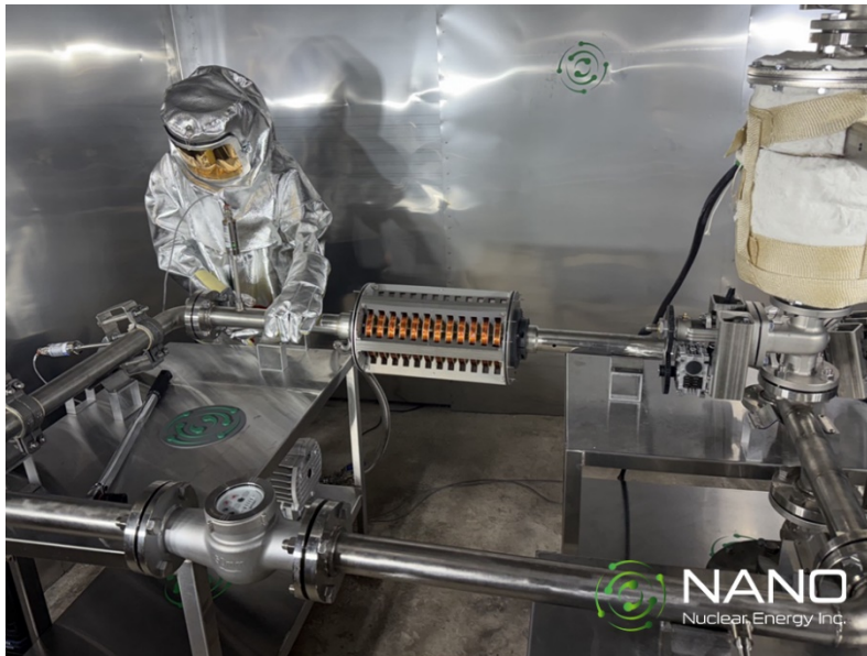
Figure 1 - NANO Nuclear Energy's ALIP Technology (center) integrated on the Test Loop inside Custom-Engineered Thermal Chamber at the Demonstration Facility in Westchester County, New York.
