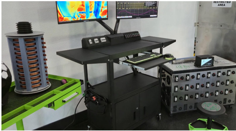
Figure 2 - ALIP's Integrated Data Acquisition System & Control Panel (ALIP pump seen at left of image)
