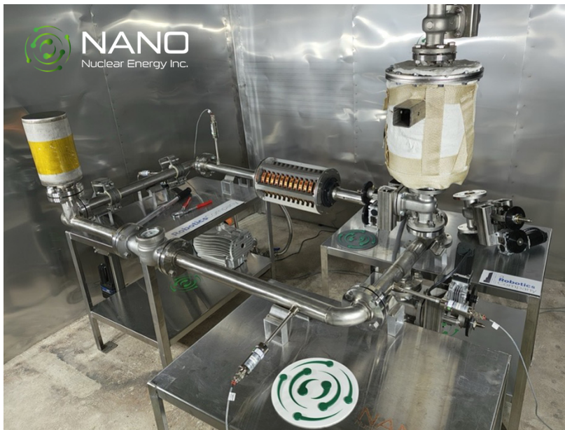
Figure 3 – ALIP (seen at center of image) Assembled Inside NANO Nuclear Energy's Custom-Engineered Thermal Chamber at the Demonstration Facility in Westchester County, New York.
