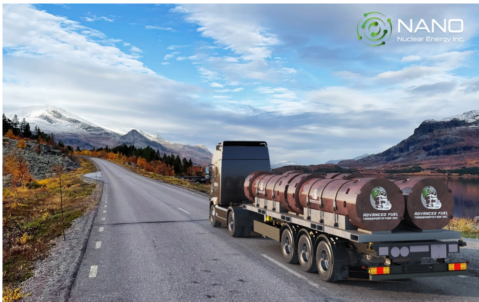
Figure 1 – Rendering of NANO Nuclear's Basket and Cask Nuclear Fuel Transportation System Being Developed in Collaboration with GNS
