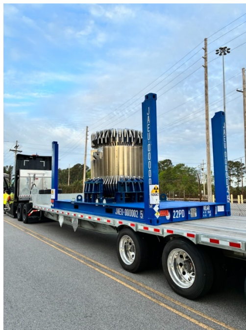
Figure 1 - A shielded industrial/nuclear radioactive material transport cask, marked with Class 7 radioactive placards and UN 3328 labels.
