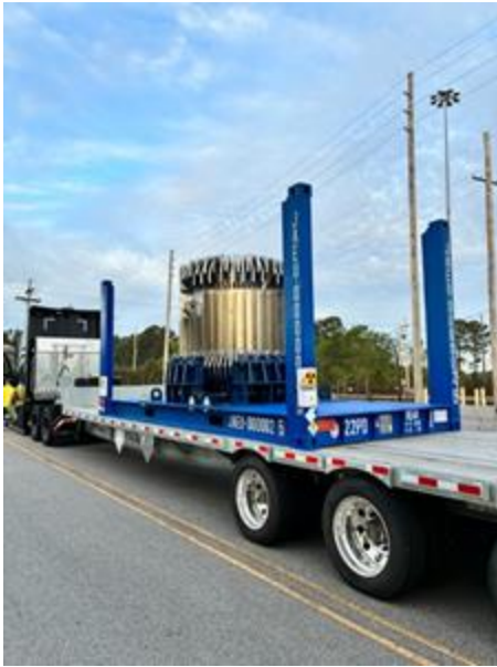
A shielded industrial/nuclear radioactive material transport cask, marked with Class 7 radioactive placards and UN 3328 labels.
